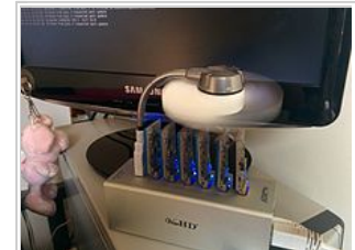
Obsolete bitcoin mining hardware called ASICMiner Block Erupter USB common in mid and late 2013. [note 14]
